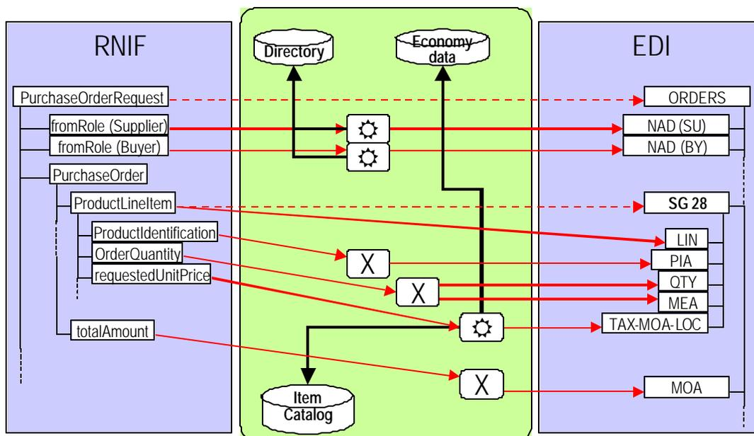
Figure 15 Message syntax mapping.
