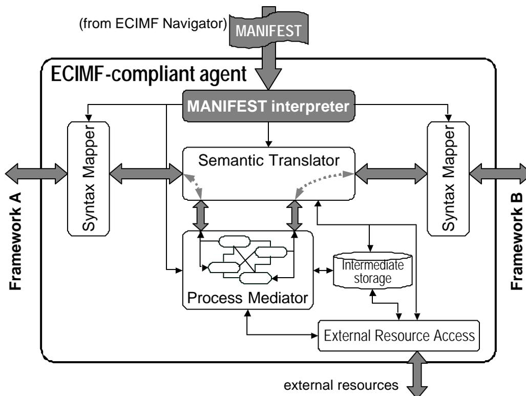
Figure 17 Example of ECIT (ECIMF-compliant agent) facilitating message exchange.
